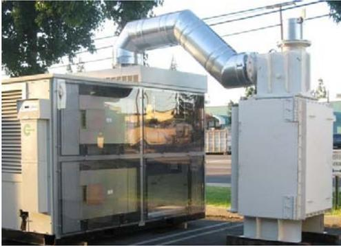
200 kilowatt (kW) natural gas-fired microturbine
